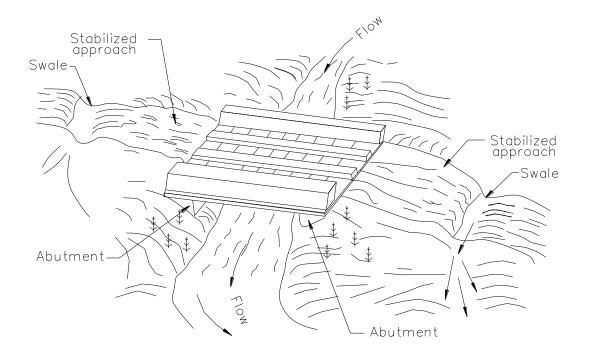
NOTE: Surface flow of road diverted by swale and/or dike.
