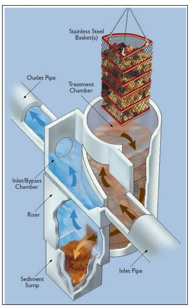
Figure 3-3 Cleansall™ Gross Pollutant Trap Schematic
