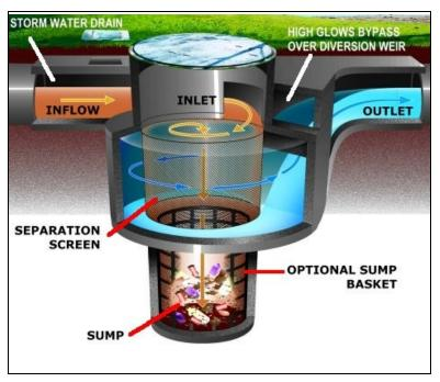
Figure 3-9 CDS<sup>™</sup> Unit Schematic
